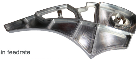
Alumina Frame Size: L1,425 x W680 x H70 mm Material: Al6061
